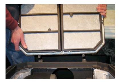
3. Use a putty knife or screwdriver to remove the old gasket. Remove any residual gasket and glue with a wire brush and vacuum.
